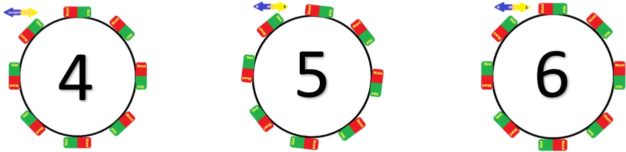
The decisive aspect is that the fixed blue-yellow switchable magnet is always switched on, exactly when it accelerates the large rotor, and is always switched off, exactly when its magnetic field would brake the large rotor.
