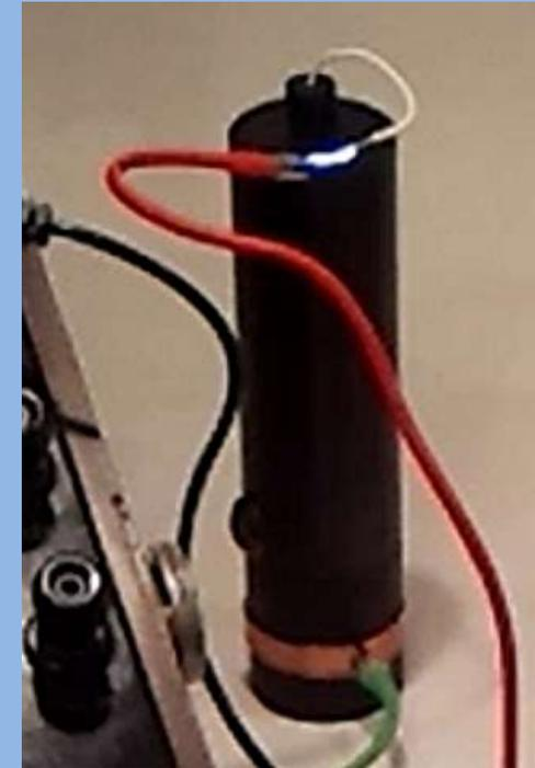
Length of the arc: 2 cm corresponding to 33 kV
